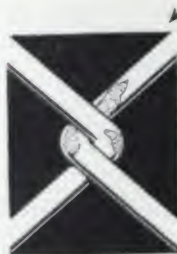
Observe how bending of pre-coated wire during weaving process causes zinc coating to crack and scale.
